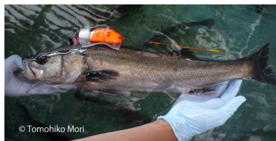
A floating package including D3GT attached to a Japanese sea bass.
